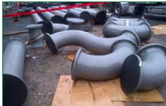
Novocoat DTM Epoxy applied on outside. Novocoat SC3300 Novolac Epoxy Lining coated inside.
