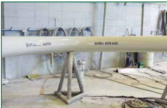
Novocoat SC2200 Rapid Set Pipe Coating applied on outside. Novocoat SC3300 Novolac Epoxy Lining applied inside.
