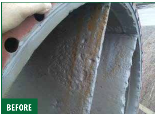
Pitted and worn steel rebuilt with Novocoat EP3900 Machinable Paste .
