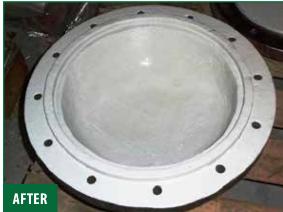
Heat exchanger floating head before and after pits in steel were filled using Novocoat EP3900 Machinable Paste . Novocoat SC5400 Lining applied as topcoat.
